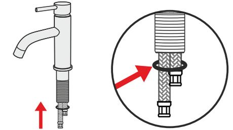
3. Place the Deck Plate (4) in position over the mounting hole in the basin. Feed the Water Inlet Hoses (9) and Threaded Pipe (5) through the Deck Plate until the Rubber O-Ring (3) and Faucet Base (2) sit on top of the Deck Plate.
