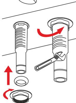
3. From underneath the drain opening, install the Drain Washer (b) onto the Pop-Up Drain (d) and then attach and tighten then the Drain Nut (c) using a wrench.
