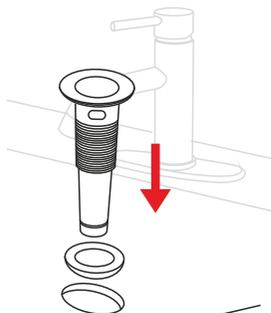
2. Place the Drain Gasket (a) on top of the drain opening and then insert the Pop-Up Drain (d) through the Drain Gasket (a) and into the drain opening.
