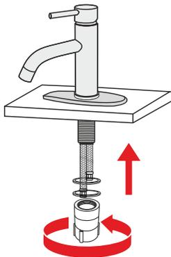
5. Connect and tighten the HOT (red) and COLD (blue) Water Inlet Hoses (9) to the hot and cold water supply. Don't overbend the hose and ensure there is no hose deformation after installation.
