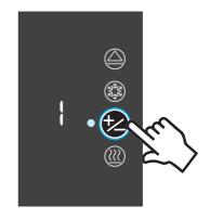
**NOTE:** Toasting can be stopped at any time by pressing the **Cancel/Eject Button.** This will cancel the operation, and the Loading Lever will move to the raised position.
